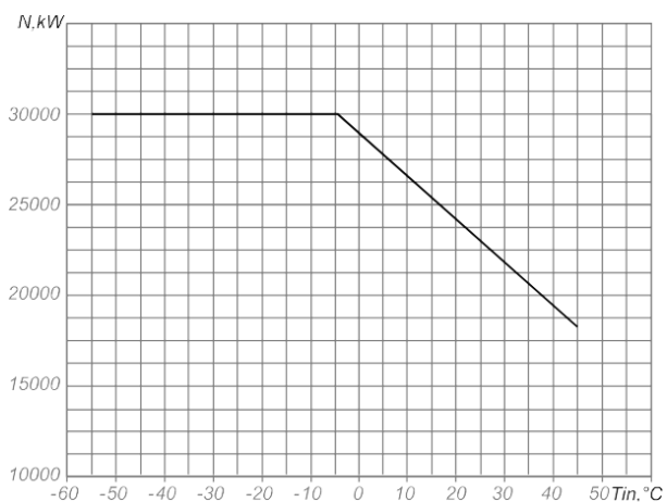
Capacity limitations of DU80L depending on air temperature at the engine's inlet
