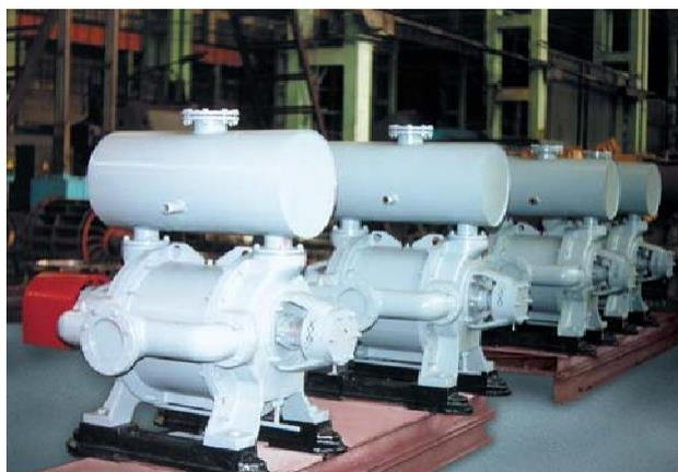
Depending on material of inner flowing part designed for pumping (creation of vacuum ) of air, inert or aggressive gases, insoluble in water, to produce or maintain vacuum. Operating medium – water.
