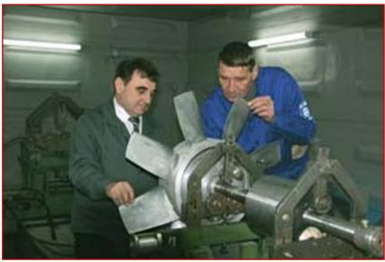
Assembly facilities incorporate 17 balancing tools that allow to perform balancing of single rotor parts and assembled rotors with diameter up to 2,100mm, length up to 4,700mm and weight up to 7,000kg. Rotation speed - up to 3,150 rpm
